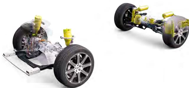
Air suspension on all four wheels gives the XC60 outstanding ride comfort – the air springs absorb up imperfections in the road – and make the car stable by keeping the ride height constant, regardless of the load. With the active chassis you can alter the way the car rides and handles to suit your mood or the road.
